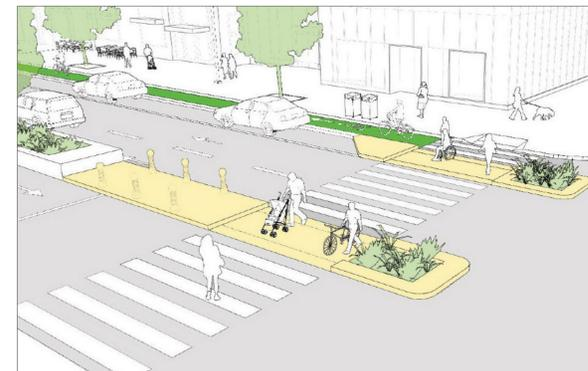
Reduces the time a pedestrian is interacting with traffic while crossing an intersection
