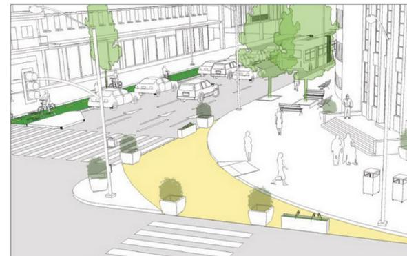
Reduces the time pedestrians interact with vehicles and allows for a single crossing point where there may have been three separate crossings
